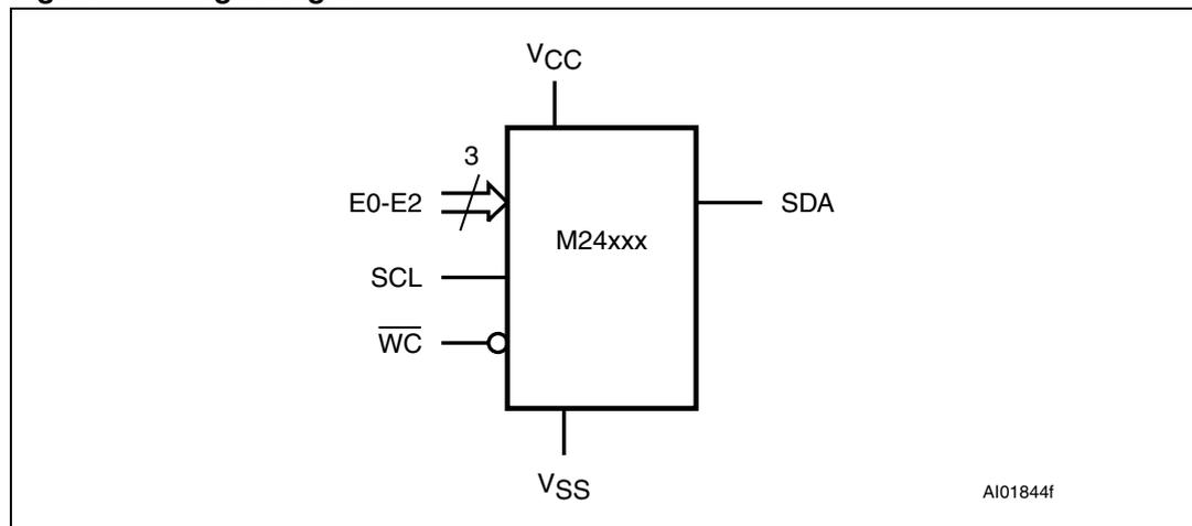
I<sup>2</sup>C uses a two-wire serial interface, comprising a bidirectional data line and a clock line. The devices carry a built-in 4-bit device type identifier code (1010) in accordance with the I<sup>2</sup>C bus definition.
