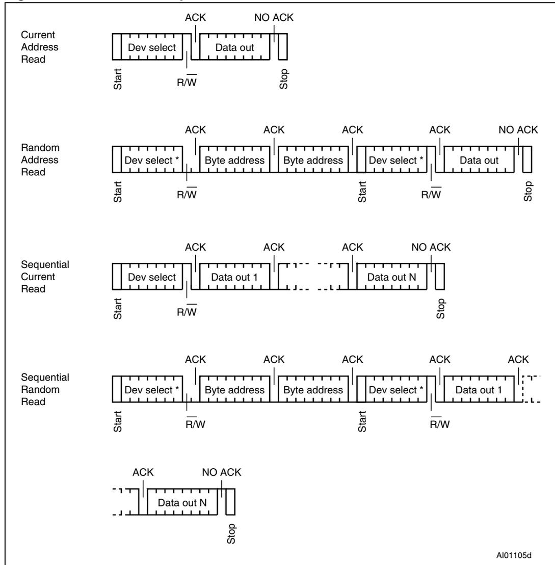
1. The seven most significant bits of the device select code of a Random Read (in the 1<sup>st</sup> and 4<sup>th</sup> bytes) must be identical.
