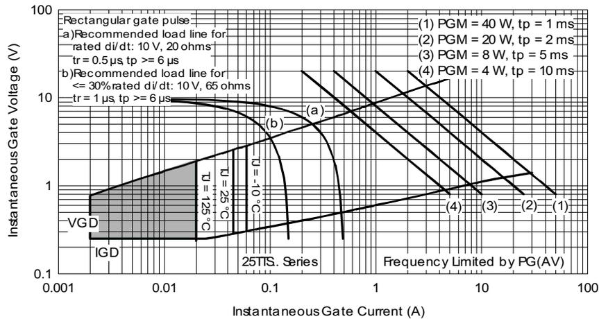
Fig. 9 - Gate Characteristics
