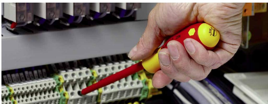
*Easily and safely, the high-quality blade insulation protects the user when working with live components.*
