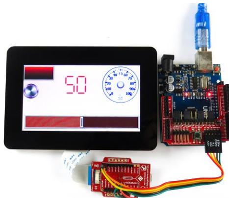
Figure 3. gen4 display (gen4-uLCD-43DCT-CLB), connected to the 4D-UPA using a 30-way FFC cable, and Jumper wires connecting to the Arduino Adaptor Shield, on top on an Arduino. This is utilising GPIO1 and GPIO2 pins, mapped through to being a different UART/COM port on the gen4 display (Diablo processor), so not to cause a conflict with the USB chip on the UPA.
