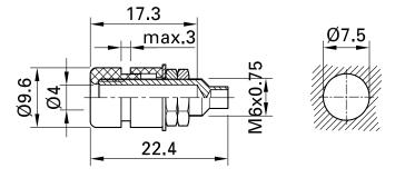
Insulated, Ø 4 mm, rigid. Machined brass. The socket can be screw-mounted in predrilled panels. Threaded bolt M6x0.75 and solder connection.
