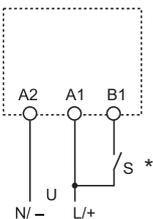
\* With DC supply, positive polarity has to be connected to B1 terminal (according to EN 60204-1).
