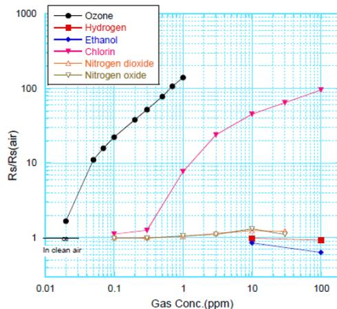
**Fig. 3 Sensitivity characteristics**
