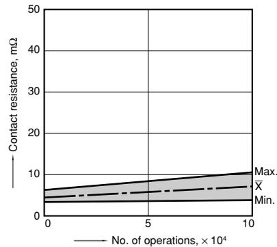
6-(3). Electrical life test (Motor lock)
