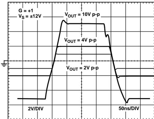
Figure 23. Large Signal Transient Response (See Figure 42)
