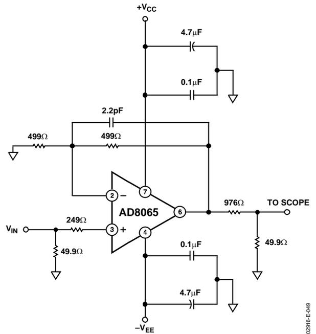
Figure 49. Settling Time
