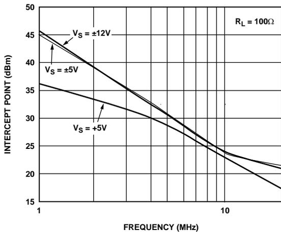
Figure 18. Third-Order Intercept vs. Frequency and Supply Voltage
