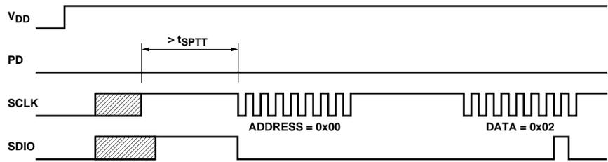
Figure 36. Power up serial port watchdog timer sequence.
