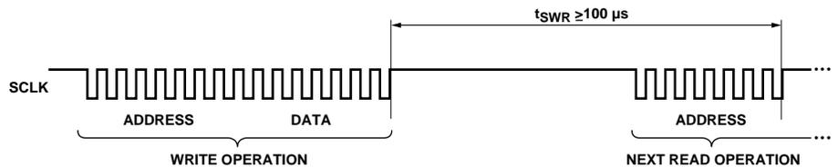
Figure 32. Timing between write and read commands.
