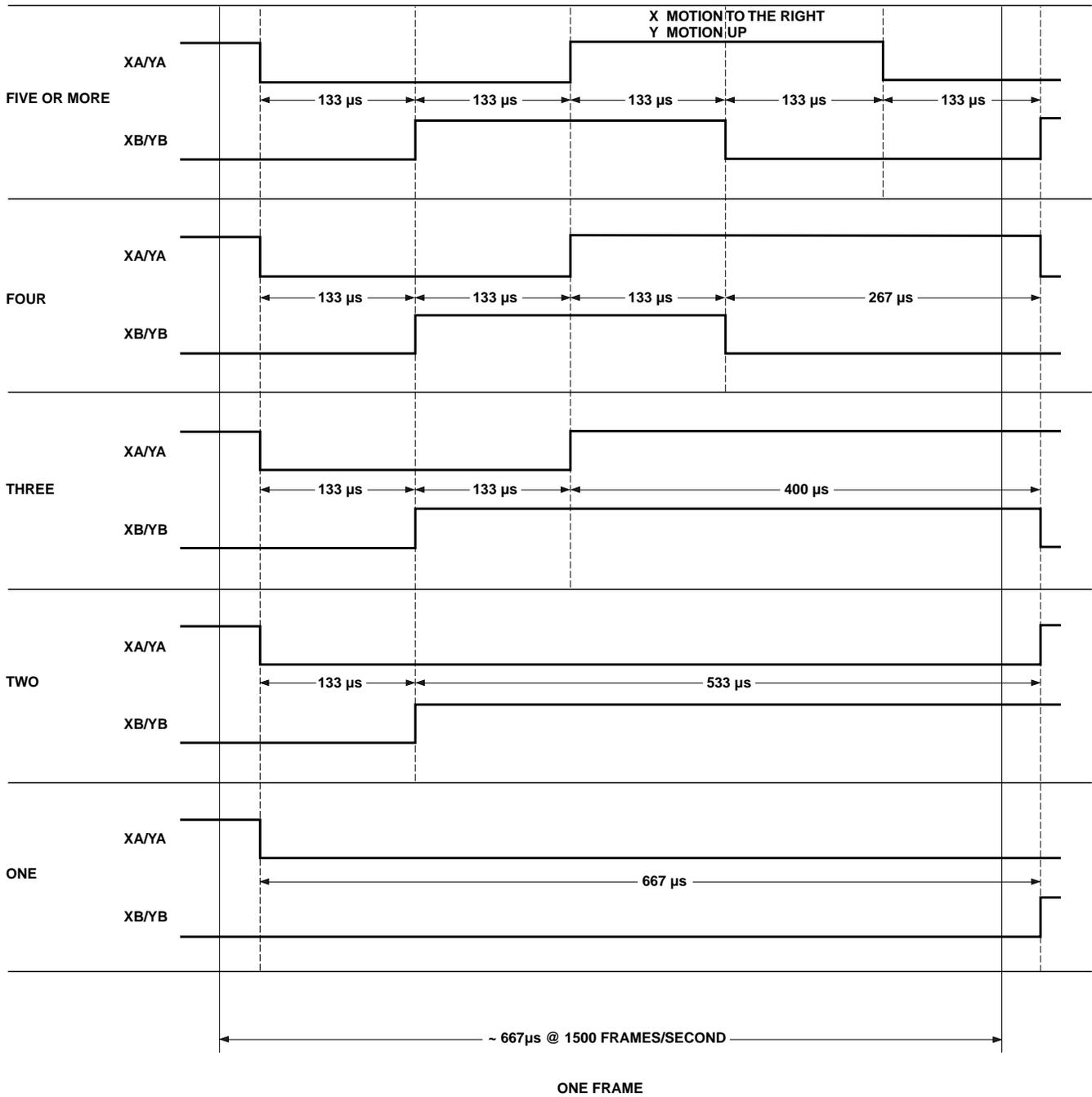
Figure 16. Quadrature states per frame (400 cpi mode).
