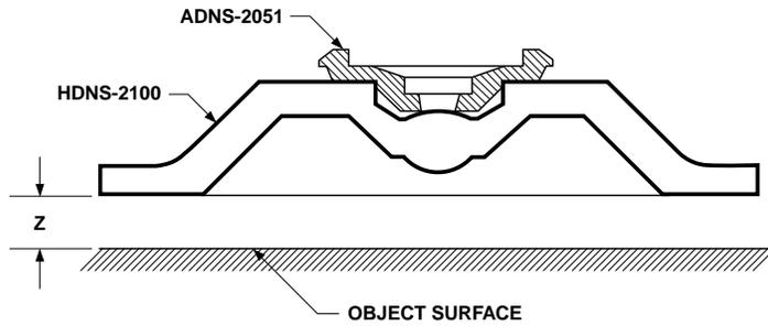
Figure 10. Distance from lens reference plane to surface.
