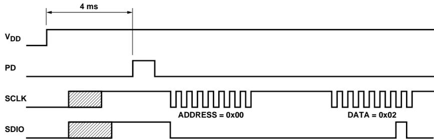
Figure 37. Power up serial port PD sync sequence.
