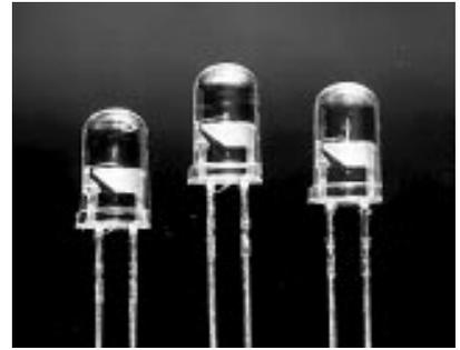
The AlInGaP II technology provides extremely stable light output over very long periods of time, with low power consumption.
