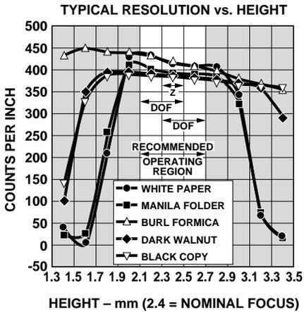
Figure 21. Typical resolution vs. Z (comparative surfaces).<sup>[2,3]</sup>
