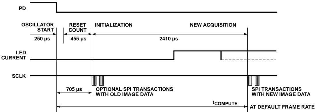
Figure 15. Detail of PD falling edge timing.
