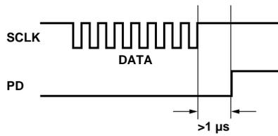
Figure 34. Timing between SCLK and PD rising edge.
