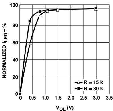
Figure 11. Typical I-V characteristic of ADNS-2051 XY\_LED pin.
