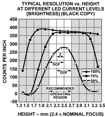
Figure 24. Typical resolution vs. z (black copy and LED variation).<sup>[2,3]</sup>
