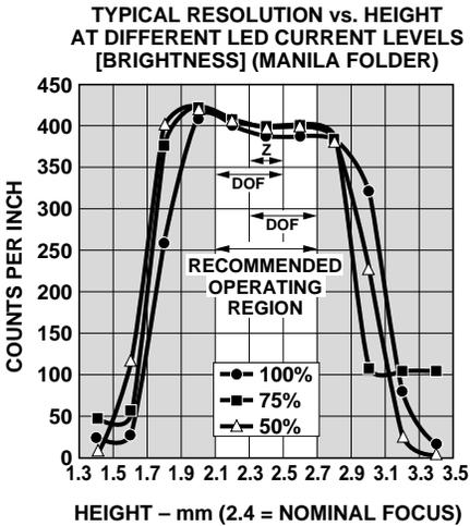
Figure 23. Typical resolution vs. z (manila folder and LED variation).<sup>[2,3]</sup>
