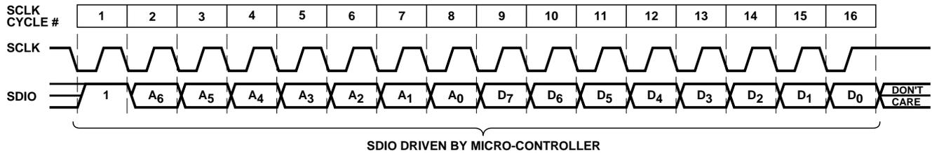
Figure 25. Write operation.
