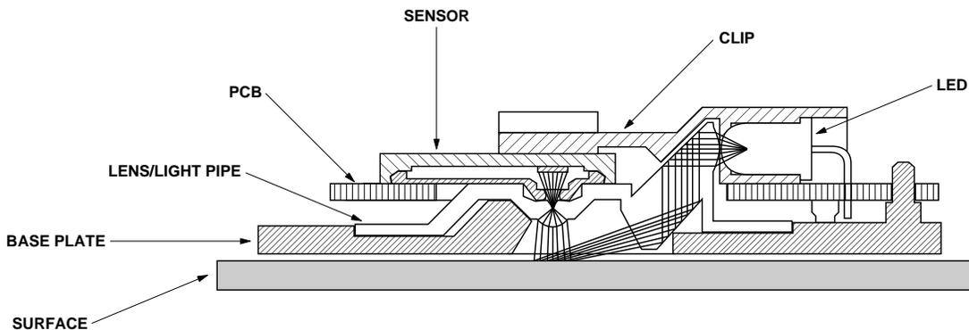
Figure 7. PCB assembly.
