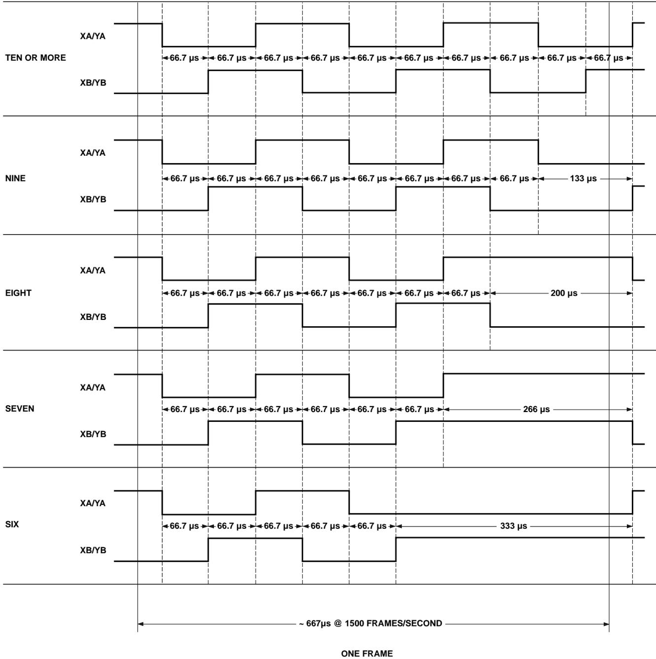
Figure 17. Quadrature states per frame (800 cpi mode).
