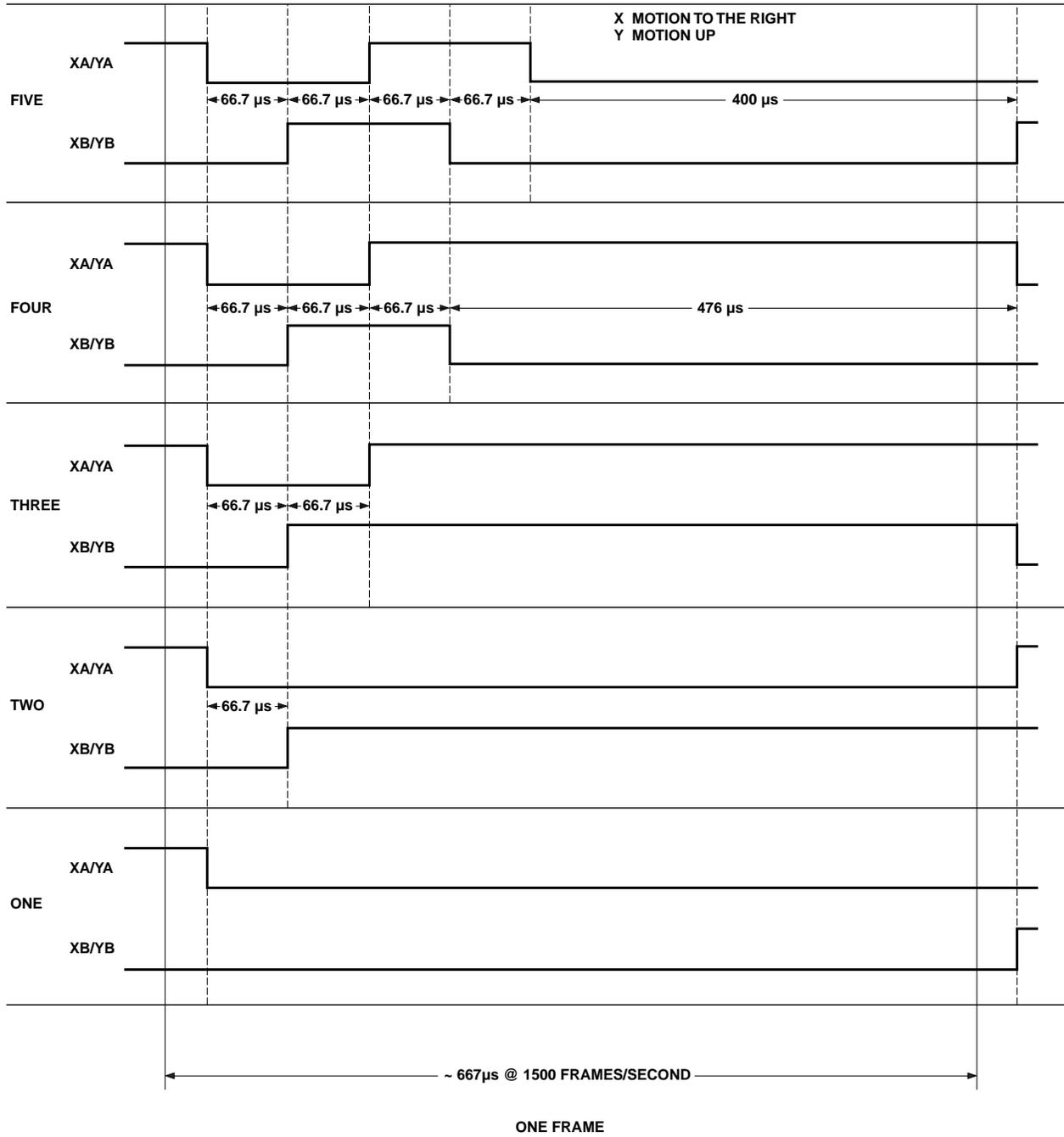
Figure 18. Quadrature states per frame (800 cpi mode).
