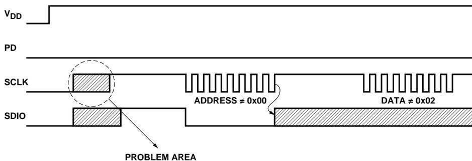
Figure 35. Power up serial port watchdog timer sequence.
