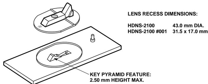
Figure 4. Illustration of base plate mounting features.
