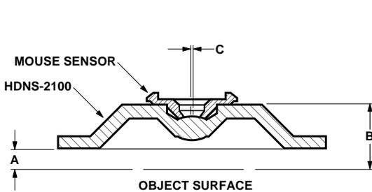
Figure 2. Optical system assembly diagram.
