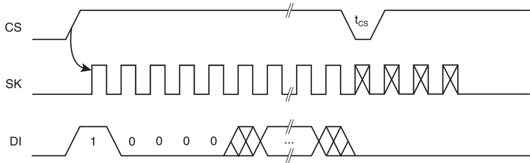
**Figure 3-5.** WRITE Timing
