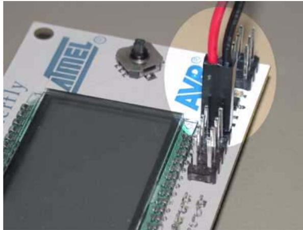
External power can be applied at pin 9 and 10 at both PORTB and PORTD, see *Figure 3-7* for the pinout.
