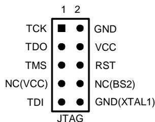
**Note:** It is highly recommended to apply external power (3,1 – 4,5V), when using the JTAG to save the battery. See Figure 3-10 for how to connect external power.
