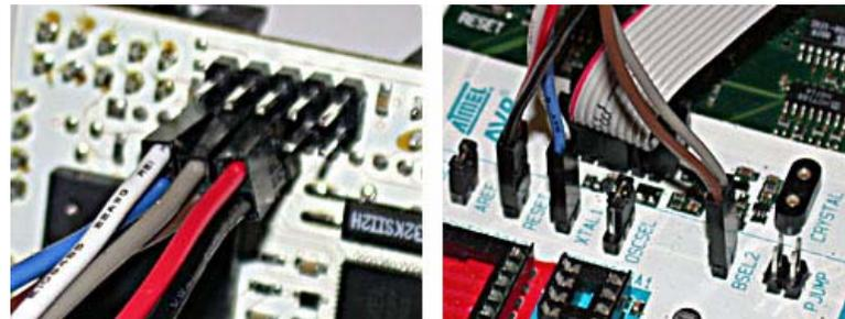
Connect PROG DATA and PROG CTRL from the STK500 to respectively PORTB and PORTD on the AVR Butterfly. Make sure that pin 1 on the STK500 connects to pin 1 on the AVR Butterfly.
