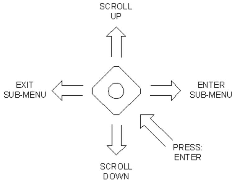
Using the joystick one can move around in the menu shown in *Figure 2-2*, and edit values, entering name, etc. Here are examples on how to enter your name.
