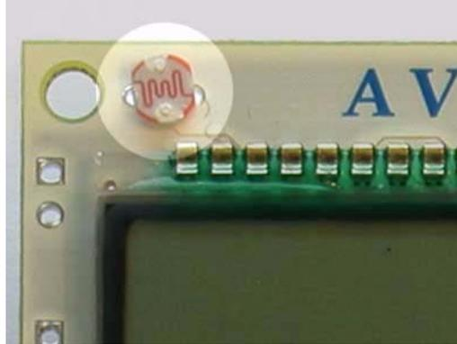
An LDR (Light Dependent Resistor) is used to measure the light. An LDR is characterised by the fact that when the light decreases the resistance goes up. Using a voltage divider and reading the voltage over the LDR through the ADC-channels on the ATmega169, the light can be calculated.
