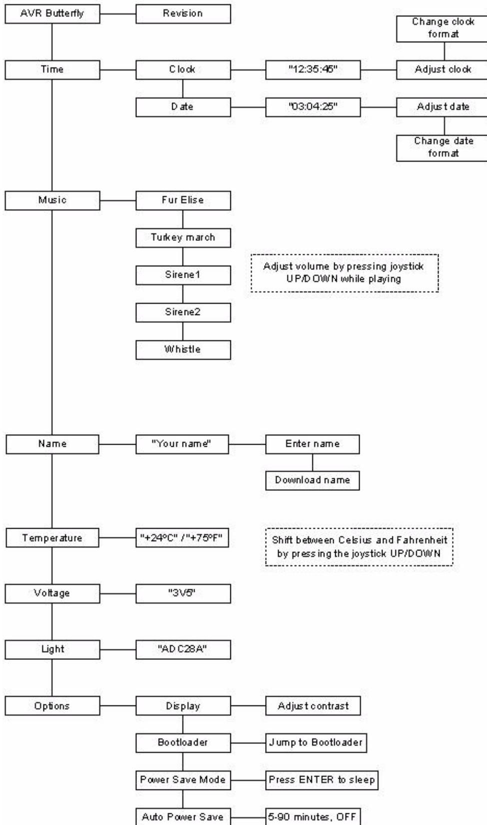
Figure 2-2 shows the menu system of the application that comes with the AVR Butterfly. The column to the left displays the main menu: “AVR Butterfly”, “Time”, “Music” etc... To shift between the alternatives in the menu, press the joystick UP or DOWN. To enter a sub-menu, press the joystick to the RIGHT. To exit a sub-menu, press the joystick to the LEFT. To enter/adjust a value, press ENTER. E.g. when “Adjust clock” appears in the LCD, press ENTER to enter the adjust function.
