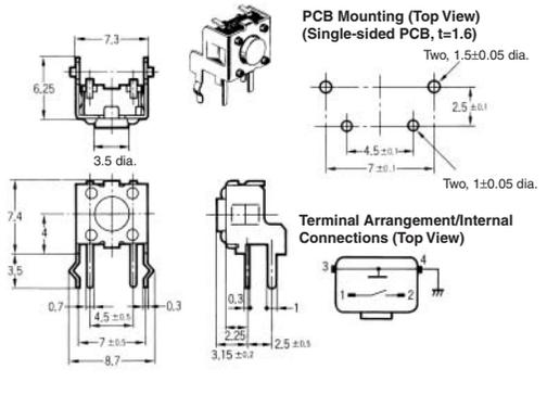
**Vertical, Flat Plunger Type (Height: 3.85 mm)**
