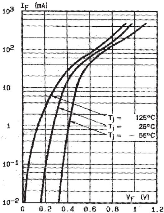
Fig. 2: Forward current versus forward voltage (typical values).
