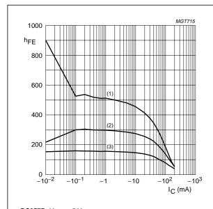
**BC857B**;  $V_{CE} = -5 \text{ V}.$
