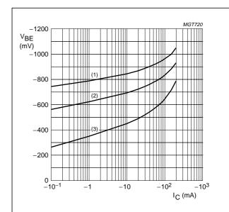
**BC857C**;  $V_{CE} = -5 \text{ V}.$
