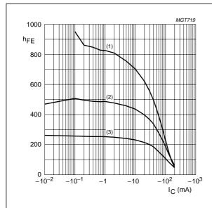
**BC857C;**  $V_{CE} = -5 \text{ V}.$
