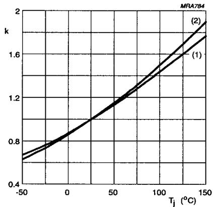
$$k = \frac{R_{DS(on)} \text{ at } T_j}{R_{DS(on)} \text{ at } 25^\circ\text{C}}$$
