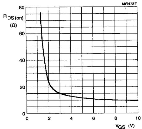
$V_{DS} = 0.1$  V;  $T_j = 25^\circ\text{C}$ .
