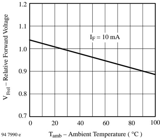
Figure 4. Relative Forward Voltage vs. Ambient Temperature
