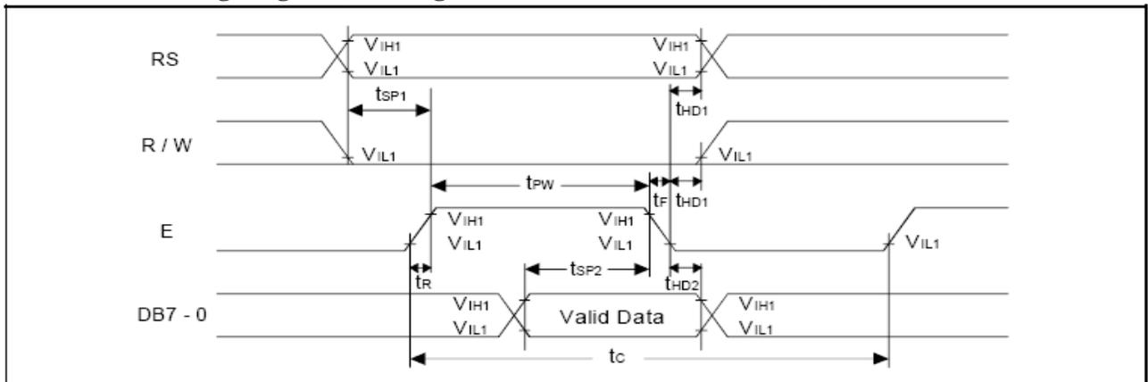
Read mode timing diagram(Reading data from SPLC780D to MPU)
