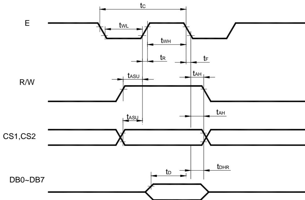
Figure 6.0 MPU Read timing
