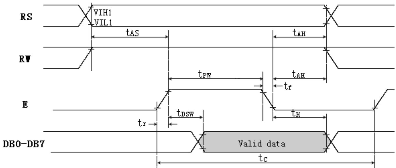
9-2-2 Read mode (reading data from ST7066 to MPU)
