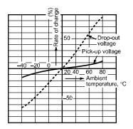
5.-(2) Change of pick-up and drop-out voltage (1 Form A 1 Form B)
