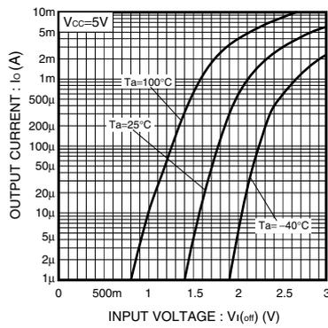
Fig.2 Output current vs. Input voltage (OFF characteristics)
