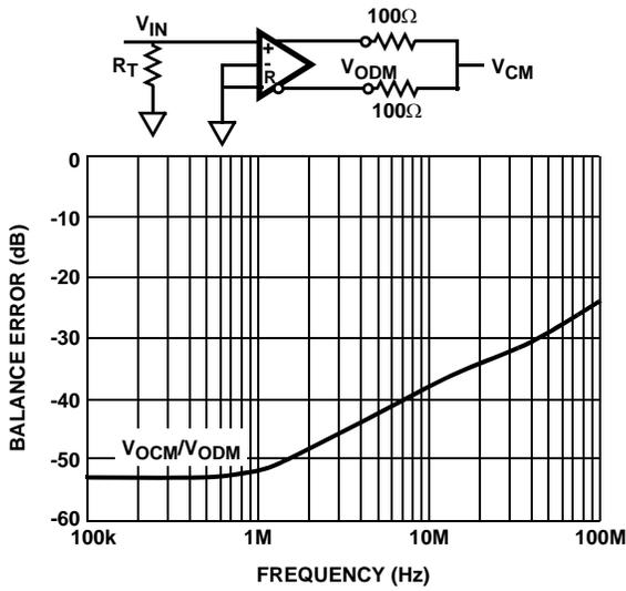
FIGURE 7. DIFFERENTIAL MODE OUTPUT BALANCE ERROR vs FREQUENCY
