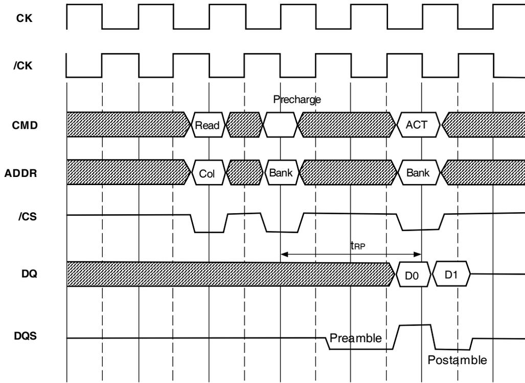
**Figure 6. Precharge Termination of a Burst Write (Burst Length=4)**
