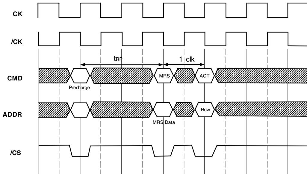
Figure 12. Active / Precharge Power Down Mode
