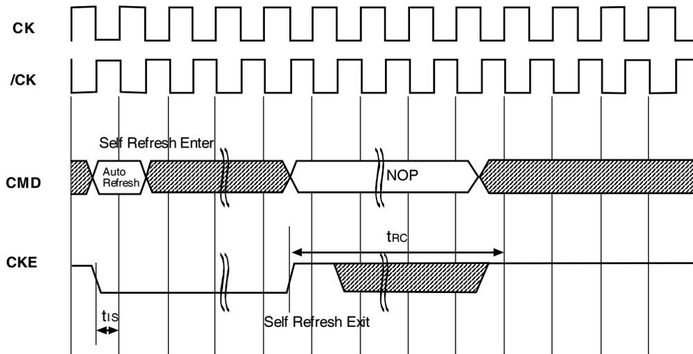
$t_{RC}$  is required before any command can be applied, and 200 cycles of clk are required before a READ command can be applied.
