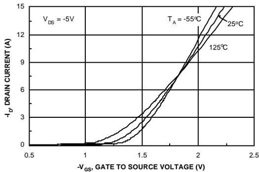
Figure 5. Transfer Characteristics.
