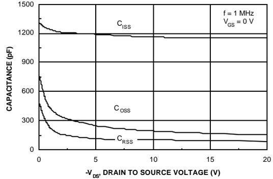
Figure 8. Capacitance Characteristics.
