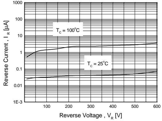
Figure 2. Typical Reverse Current vs. Reverse Voltage
