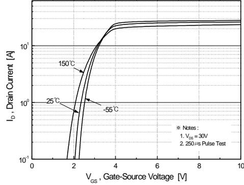
**Figure 2. Transfer Characteristics**
