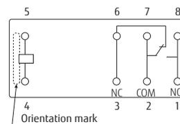
Connect terminal #1 and #8 on the PC board
