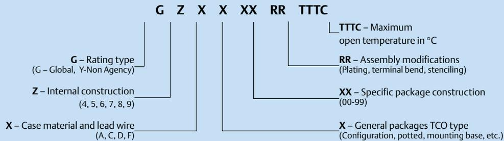
As shown above, Therm-O-Disc MICROTEMP® TCOs follow a consistent product nomenclature that identifies the basic product type, lead wire size, special features and packaging options. For example, a standard G4 series TCO calibrated to open at 192°C would have a part number G4A00192C.
