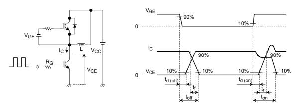
Note 2: Switching loss measurement waveforms
