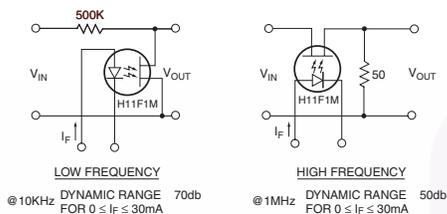
Distortion free attenuation of low level A.C. signals is accomplished by varying the IRED current,  $I_F$ . Note the wide dynamic range and absence of coupling capacitors; D.C. level shifting or parasitic feedback to the controlling function.
