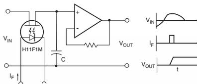
Accuracy and range are improved over conventional FET switches because the H11FXM has no charge injection from the control signal. The H11FXM also provides switching of either polarity input signal up to 30V magnitude.
