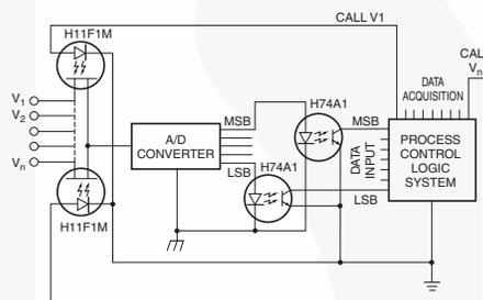
The optical isolation, linearity and low offset voltage of the H11FXM allows the remote multiplexing of low level analog signals from such transducers as thermocouples, Hall effect devices, strain gauges, etc. to a single A/D converter.
