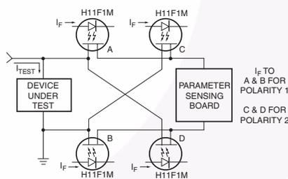
In many test equipment designs the auto polarity function uses reed relay contacts to switch the Kelvin Contact polarity. These reeds are normally one of the highest maintenance cost items due to sticking contacts and mechanical problems. The totally solid-State H11FXM eliminates these troubles while providing faster switching.
