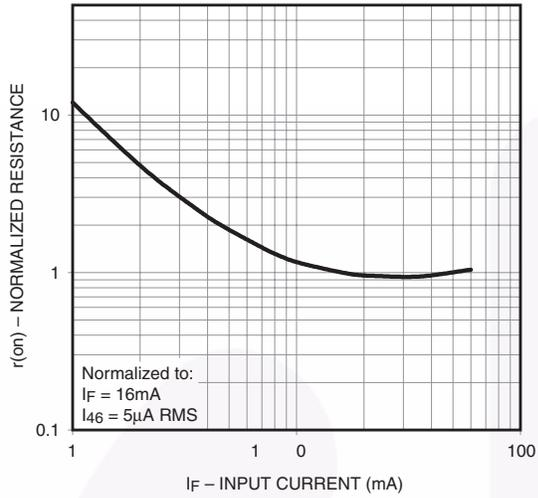
Figure 2. Output Characteristics
