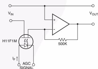
This simple circuit provides over 70db of stable gain control for an AGC signal range of from 0 to 30mA. This basic circuit can be used to provide programmable fade and attack for electronic music.
