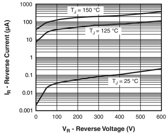
Fig. 2 - Typical Reverse Current vs. Reverse Voltage
