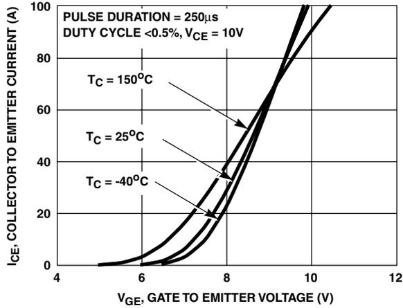
FIGURE 1. TRANSFER CHARACTERISTICS
