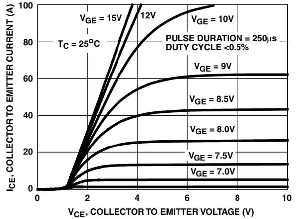
FIGURE 2. SATURATION CHARACTERISTICS
