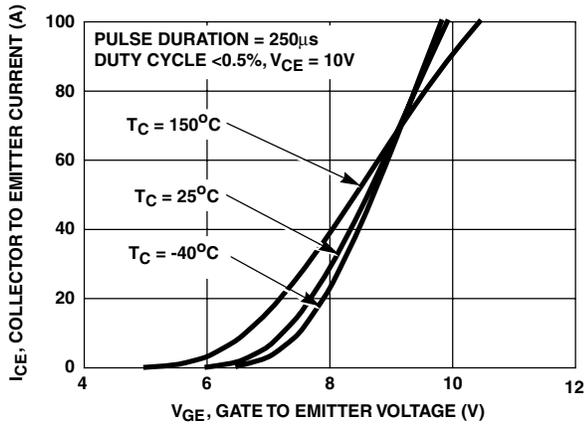
FIGURE 1. TRANSFER CHARACTERISTICS
