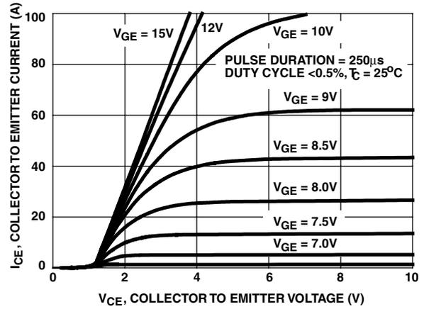
FIGURE 2. SATURATION CHARACTERISTICS
