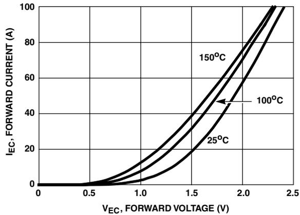
FIGURE 16. DIODE FORWARD CURRENT vs FORWARD VOLTAGE DROP
