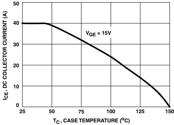
FIGURE 3. DC COLLECTOR CURRENT vs CASE TEMPERATURE
