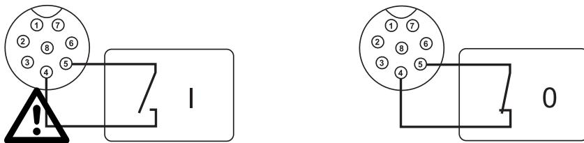
**No voltage must be applied to contacts 4 and 5.**
