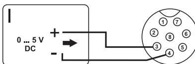
**The voltage on the remote control connection must not exceed 5V.
