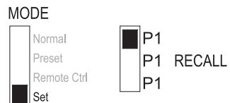
Select the respective memory slot "P1, P2 or P3" on the rear "RECALL" (15) slider. The respective values for current and voltage are indicated on the display (2/3).
