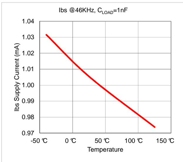
**Figure 13: I<sub>BS</sub> Current @1nF Load vs. Temperature**
