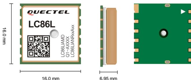
The LC86L is an ultra-compact GNSS module with an integrated patch antenna and a GNSS chipset engine that achieves perfect performance by supporting two GNSS constellations (either GPS + GLONASS or GPS + BeiDou) and QZSS. The module boasts 33 tracking channels, 99 acquisition channels, and 210 PRN channels, and it is compatible with Quectel GPS module L80 and GNSS module L86.
