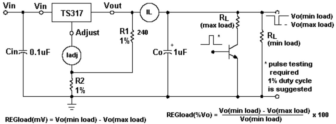
Figure 2. load regulation and  $\Delta I_{adj}/line$  test circuit
