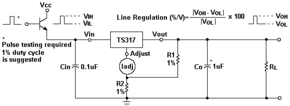
Figure 1. line regulation and  $\Delta I_{adj}/\text{line}$  test circuit
