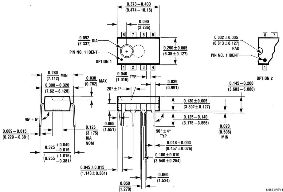
**8-Lead (0.300" Wide) Molded Dual-In-Line Package**
