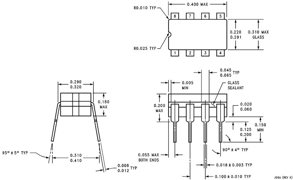
**8-Lead Ceramic Dual-In-Line Package**
