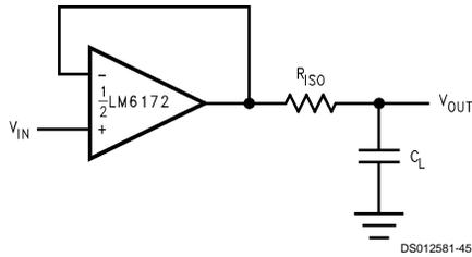
FIGURE 1. Isolation Resistor Used to Drive Capacitive Load
