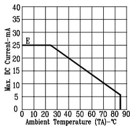
Fig8. MAX. ALLOWABLE DC CURRENT VS. AMBIENT TEMPERATURE.
