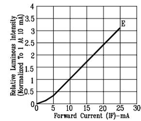
Fig3. RELATIVE LUMINOUS INTENSITY VS. FORWARD CURRENT
