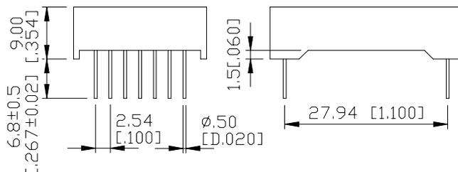
NOTES: All dimensions are in millimeters. Tolerance is  $\pm 0.25$  mm (0.01") unless otherwise noted.
