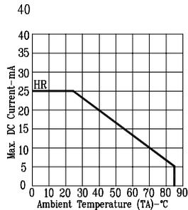
Fig5. MAX. ALLOWABLE DC CURRENT VS. AMBIENT TEMPERATURE.
