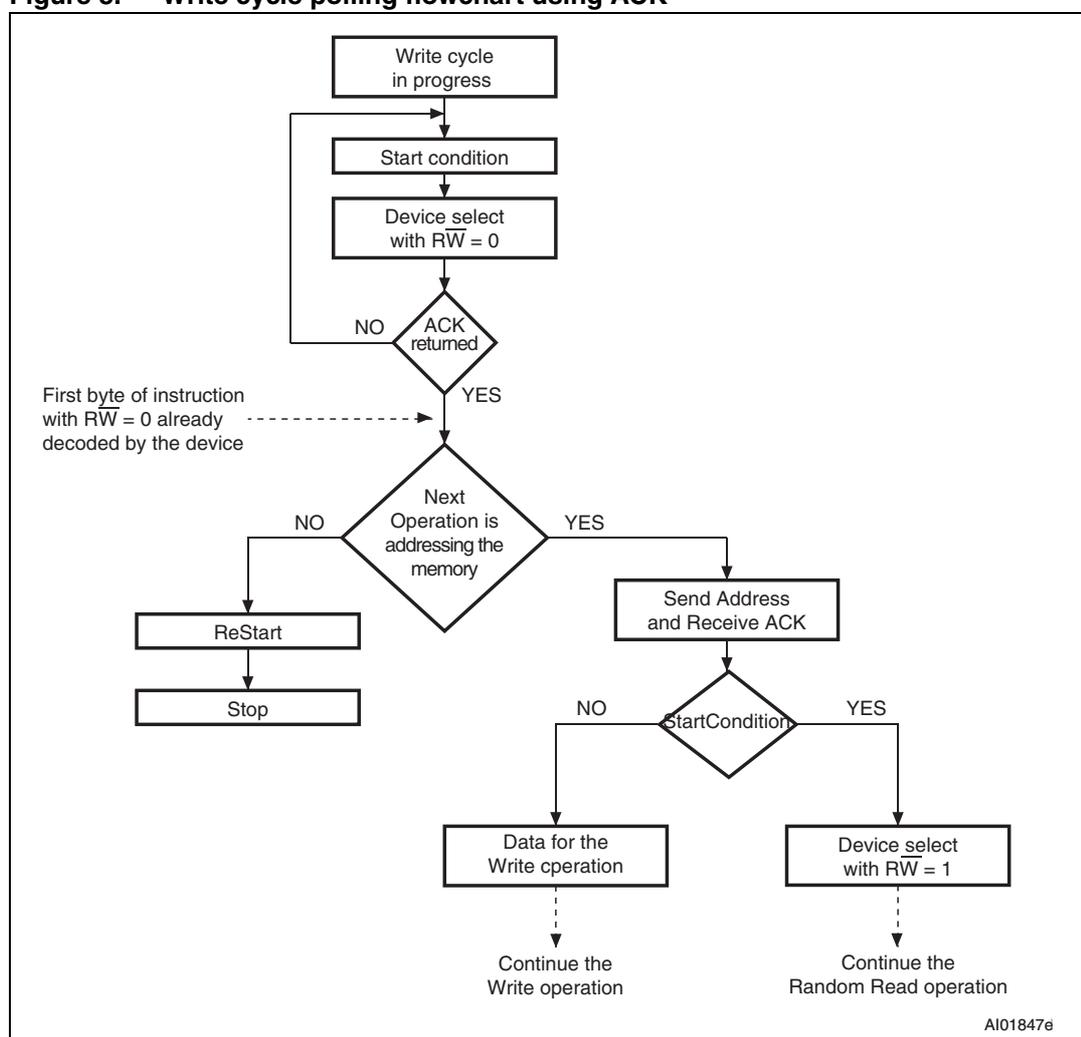
1. The seven most significant bits of the Device Select code of a Random Read (bottom right box in the figure) must be identical to the seven most significant bits of the Device Select code of the Write (polling instruction in the figure).
