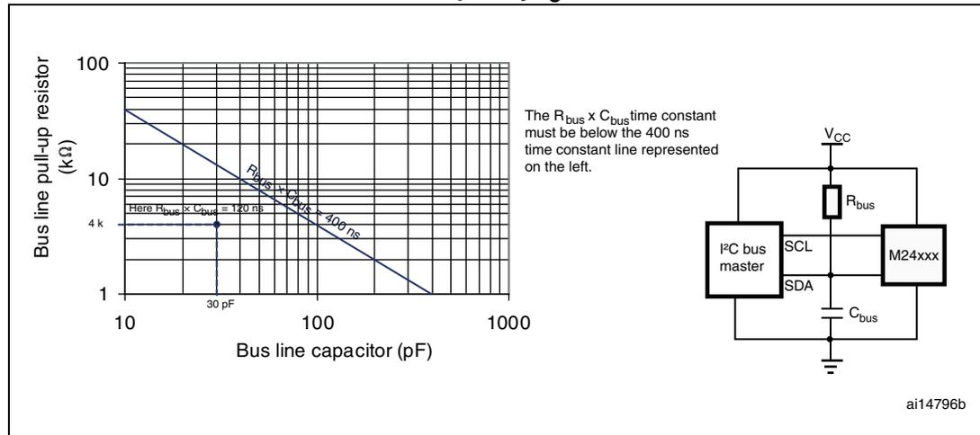
**Figure 12. Maximum  $R_{bus}$  value versus bus parasitic capacitance  $C_{bus}$ ) for an I<sup>2</sup>C bus at maximum frequency  $f_C = 1$  MHz**
