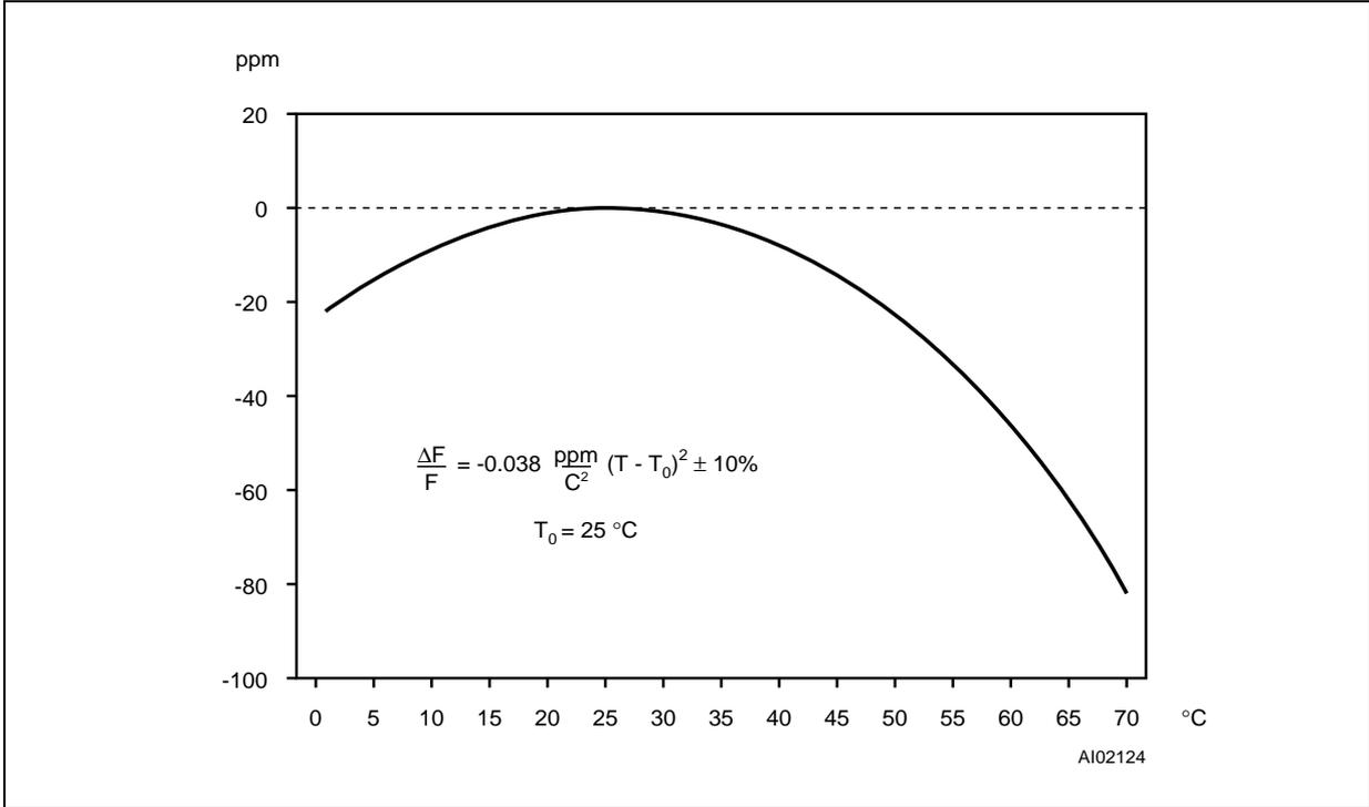
Figure 11. Clock Calibration
