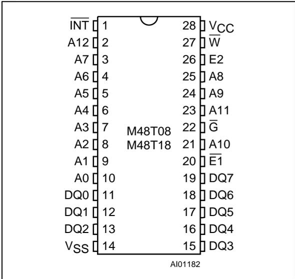
Figure 5. SOIC Connections
