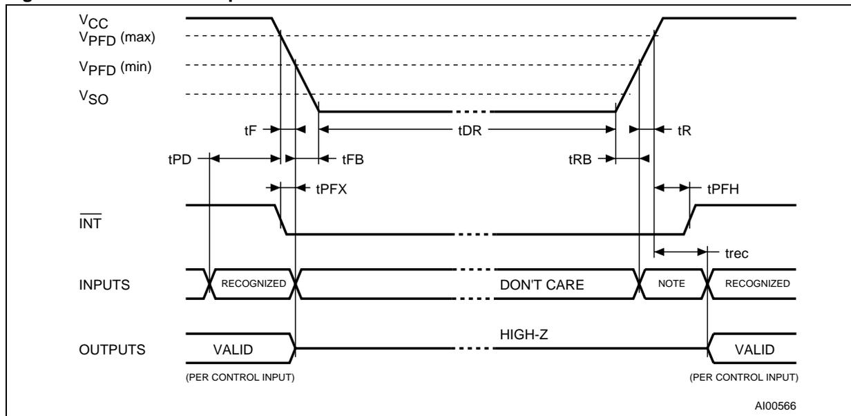
Note: Inputs may or may not be recognized at this time. Caution should be taken to keep  $\overline{E1}$  high or E2 low as  $V_{CC}$  rises past  $V_{PPFD}(\min)$ . Some systems may perform inadvertent WRITE cycles after  $V_{CC}$  rises above  $V_{PPFD}(\min)$  but before normal system operations begin. Even though a power on reset is being applied to the processor, a reset condition may not occur until after the system clock is running.
