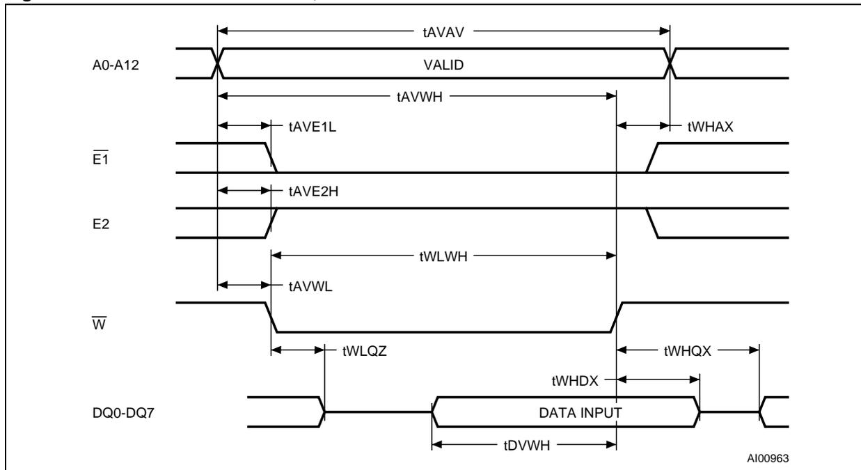
Figure 9. Chip Enable Controlled, WRITE AC Waveforms
