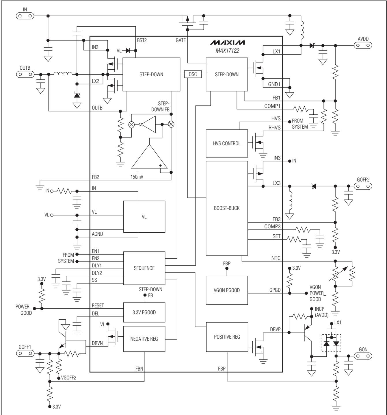
Figure 2. Functional Diagram
