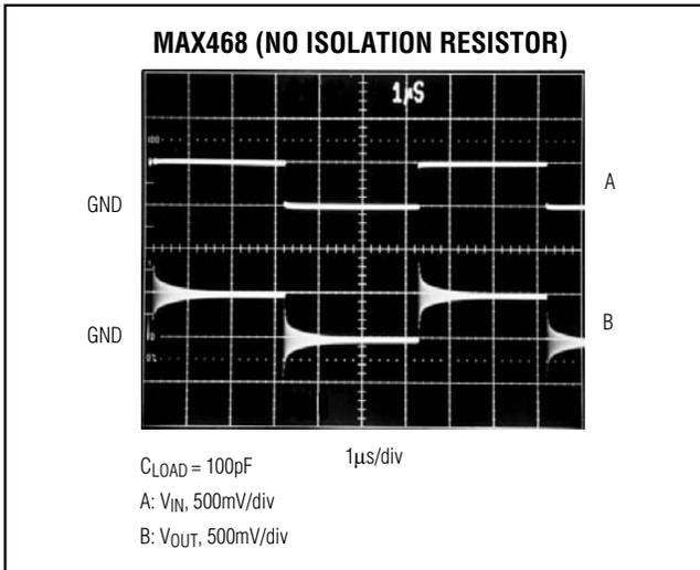
Figure 3b. Step Response without an Isolation Resistor
