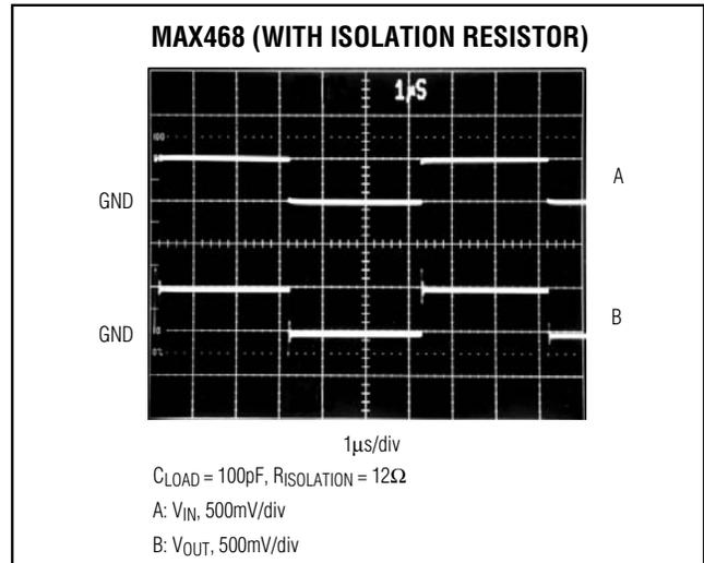
Figure 3c. Step Response with an Isolation Resistor
