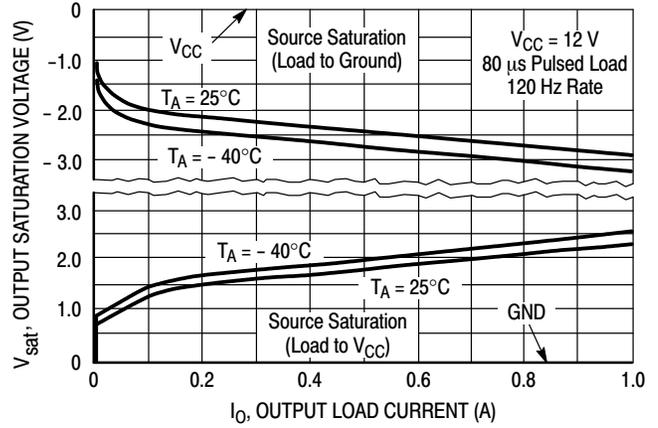
Figure 9. Drive Output Saturation Voltage versus Load Current
