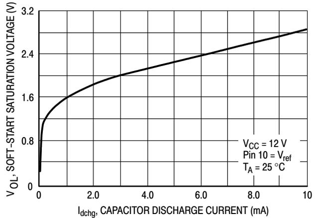
Figure 11. Soft-Start Saturation Voltage versus Capacitor Discharge Current
