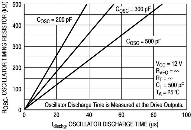
Figure 2. Oscillator Timing Resistor versus Discharge Time
