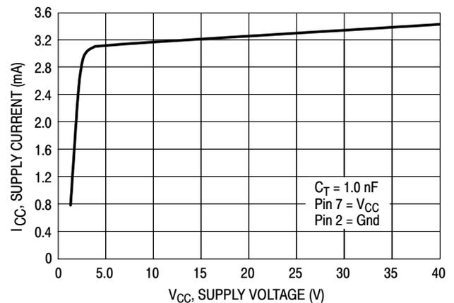
Figure 7. Standby Supply Current versus Supply Voltage
