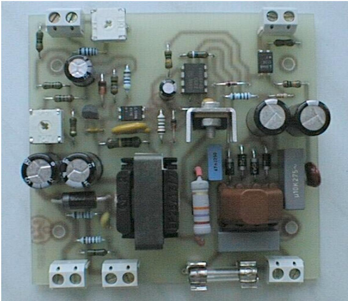
As it is well known, according to power saving regulations, we need to obtain a very low power consumption during standby condition for all equipment continuously powered on the mains. For “not saving” version of power supply, the standby power consumption is around 9.0 W (for 100 W power output). When using the MC44608 GreenLine™ Power supply controller, we obtain 1.3 W in standby mode. The result is absolutely phenomenal, but still, for some special applications, the
