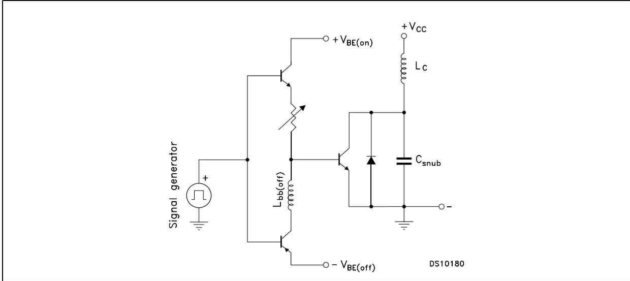
Figure 12. Reverse biased safe operating area test circuit
