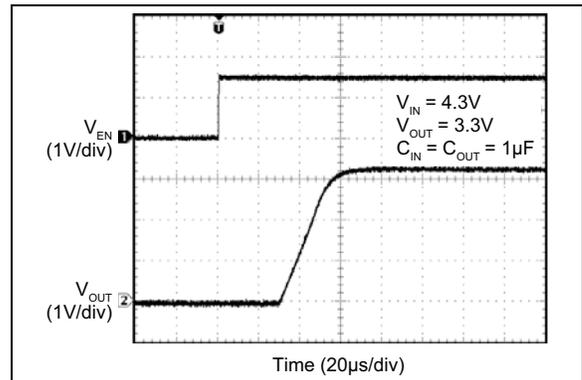
**FIGURE 2-12:** Enable Turn-On.
