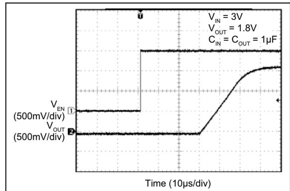
**FIGURE 2-11:** Enable Turn-On.
